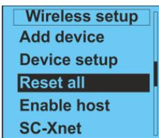
Clears all pairing and configurations. Reconfigures the radio channel to a random value.
